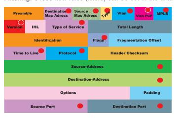
The red dot marked fields can be used as a match for a packet, stand-alone, combined or with wild cards. For IP Src and IP Dst super nets are supported.
