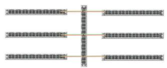
In this application 6 EX 32100 are connected to a central with 186 available 100 Gbit ports (31 per box).
