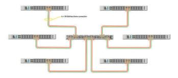
6 x EX20400 are connect over 4 x 100 Gbit to one EX 32100 to build a 500 port 10 Gbit cross connect.
