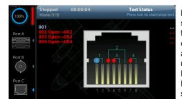
Metro.Cable can measure cable length, distance to faults, for coaxial, twisted pairs that are being used in Ethernet installations using RJ45 twisted pairs and E1, TV or any other installations using BCN.
